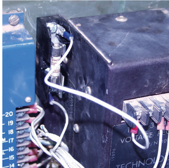
Figure 4 Top Wire Connection
